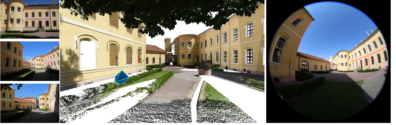
Figure 8: Lidar laser scan for testing our pose estimation algorithms with a 3-perspective-1-omnidirectional multi-view camera system. The extracted 2D lines are shown on the 2D images, while on the Lidar scan (middle) red dots are the estimated positions and green dots are the real location of the markers in metric 3D space.
