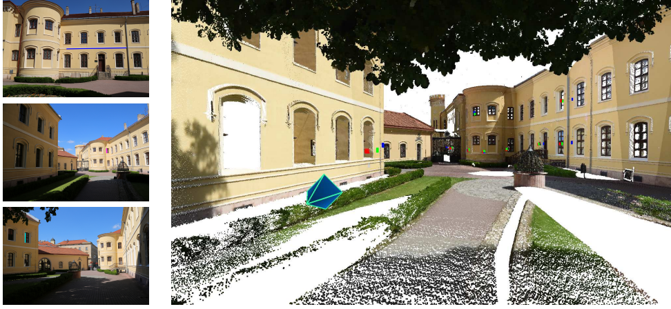
Figure 9: Lidar laser scan for testing our pose estimation algorithms with a 3-perspective camera system. The extracted 2D lines are shown on the 2D images (left). On the Lidar scan (right), red dots are the estimated positions of our minimal solver, blue dots are the estimated positions of NP3L [16], and green dots are the real location of the markers in the 3D metric space.
